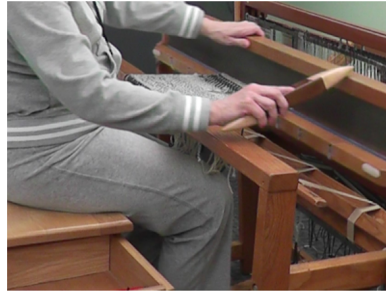
Fig. 8. Jen, a novice blind weaver, holds shuttle with right hand and prepares to pull beater with left hand.
