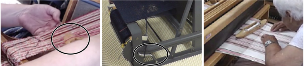
Fig. 2. Examples of common situations considered mistakes by weavers. On the left, weaver passes shuttle in between warp threads rather than through the shed. Middle image depicts a piece of weft yarn caught in a component of the loom. On the right, weaver detects a disruption in the woven pattern as a result of following an unintended weaving sequence.
